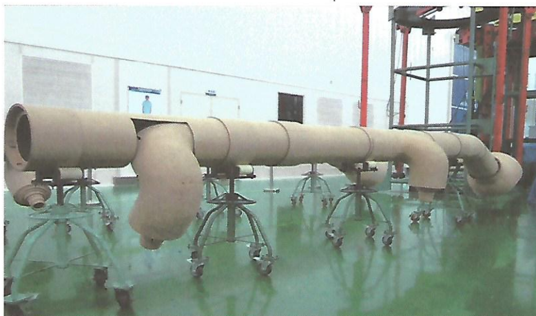
The insulation outlet device for converter transformer
